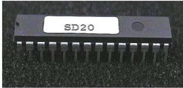
The SD20 chip is a pre-programmed PIC16F872 running at 8MHz. Position commands for up to 20 servo's are sent to the chip over the I2C bus.
